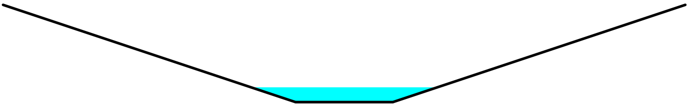
Reach 14R: Roadside Swale
